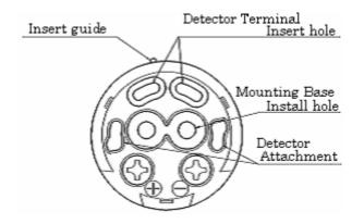
Conformity wire 18-26AWG (Incase of Pin terminal, under  $\phi 2mm$ ) Strip length  $4\sim 5mm$
