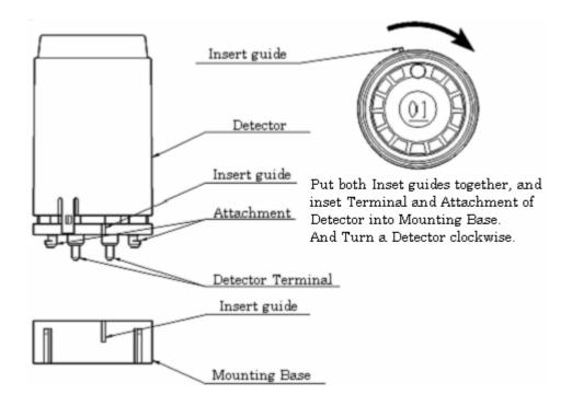
Please put both insert guides together, and insert Terminal and Attachment of Detector into Mounting Base. And Turn a Detector Clockwise until make a sound with "a snick". (See above)
